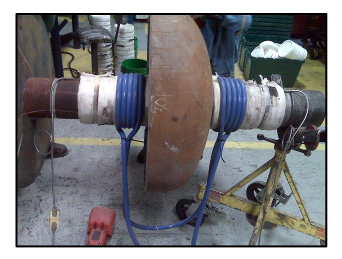
A large diameter cylinder end cap requires preheat at both weld locations on a steel shaft. This is often done by forming two coils with one heating cable, using part of the cable to bridge over to the opposite side.
