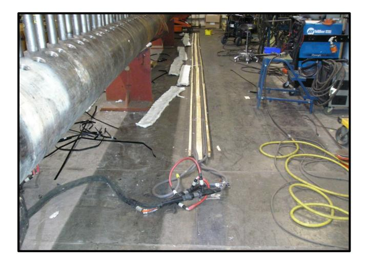
The 140 ft. (43 m) liquid-cooled heating coil is ideal for creating an elongated coil to preheat long parts such as this header, or long seam welds common when welding plate together. Once again, strongly promote the use of the tested, woven silica insulation, not KAOWOOL or fiberglass insulation that customers try to use to save money. Other untested materials may not have the insulating properties needed to protect the heating cable.
