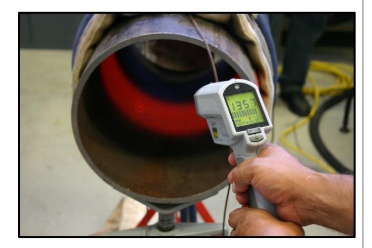
Temperatures are very uniform using induction heating coils from 12 o'clock to 6 o'clock on a test pipe.
