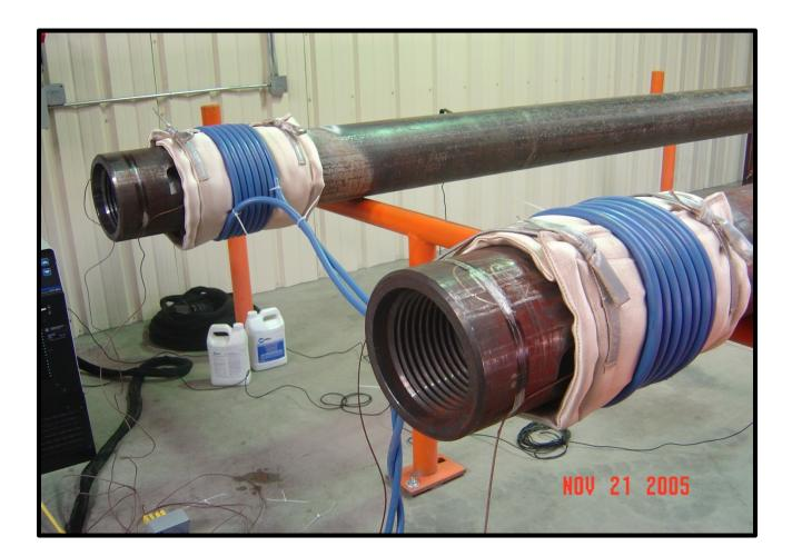
More than one location can be heated easily with one heating cable if the part geometry is the same, and the temperature requirements are the same. In this PWHT application, similar drill pipe weldments are being heated using one PROHEAT output cable and one heating cable. Although not shown here, pipe caps or end plugs should be used whenever possible to help retain heat.
