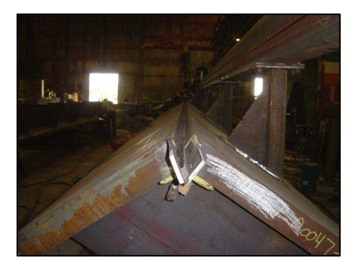
Another view of the thick plate preheat application showing the blanket underneath the steel and secured by the wood board. This is a sub-arc (SAW) welding application with run-off tabs tacked to each end of the long plates. Two ProHeats were used in this application, maintaining preheat temperatures continuously for 12 hours.
