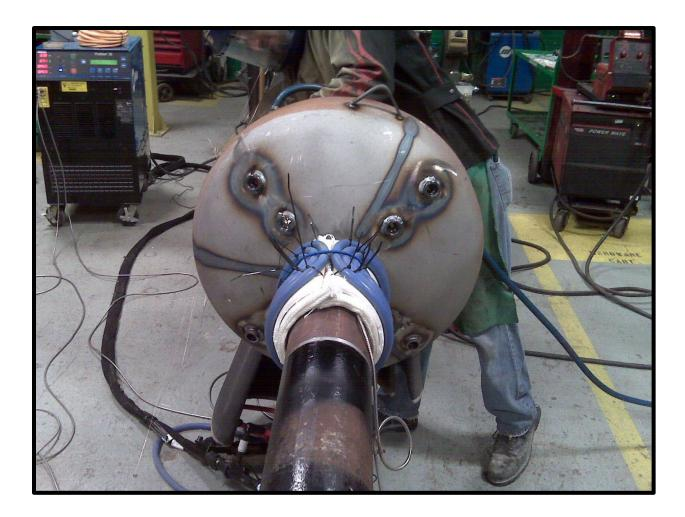
Instead of a spiral coil around the pipe, two elongated pancake coils were used to consider the possibility of using a clam shell fixture to easily install and remove the coil. Ease of use often dictates what kind of coil to try.
