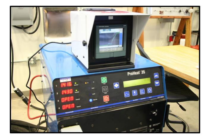
This is a high temperature PWHT application common for 9% chrome alloy piping showing two thermocouple readings above 1400 F (760 C). Note that the recorder has documented the controlled heating rate up to the soak temperature as well as the very tight temperature control during soak.
