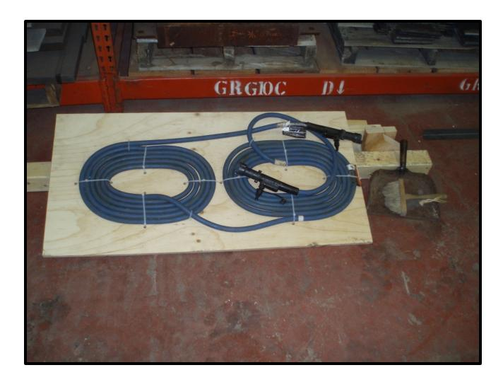
Using one heating coil, a double turn "pancake" style coil is being laid out for preheat testing in front of a moving subarc torch. The PROHEAT is capable of heating 1" (25 mm) thick steel to over 250 F (121 C) preheat temperatures while moving at typical weld travel speeds.
