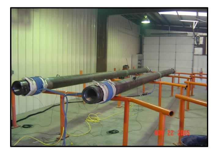
This is another drill pipe application where 4 locations are being heated at the same time using two PROHEAT output cables and 2 heating cables. It is important that the geometry and temperature requirements are the same when using both of the PROHEAT's outputs, because there is no independent control of each.
