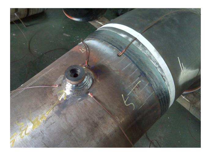
All PWHT applications require temperature feedback to control power source output for heating rates and soak temperature requirements called out in the specifications. The number of thermocouples and their locations are usually specified in the PWHT procedure.
