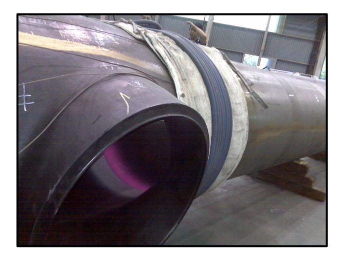
A large diameter P91 pipe requires localized stress relief at the weld. **ALWAYS** suggest to your customers that additional insulation **AND** plugging the pipe ends will improve the heating rates and the chance for successfully heating to soak temperatures called out by the procedure.
