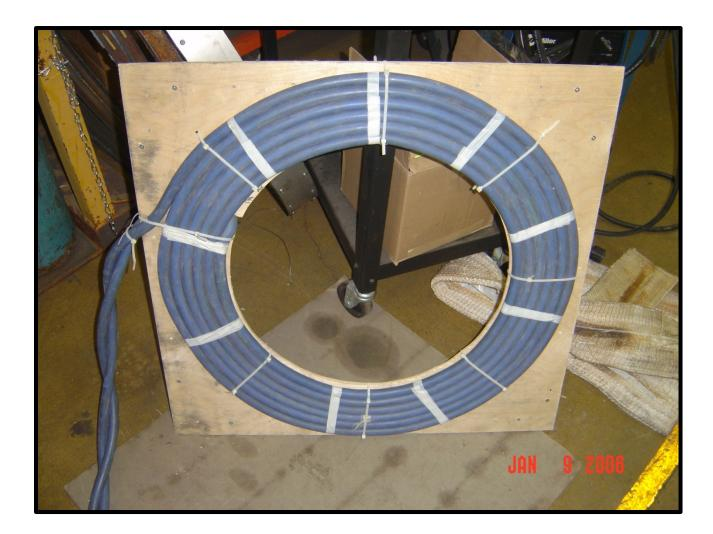
This round, but flat "pancake" coil was created for a preheat application where a thin-wall pipe was being welded to a thick, circular base plate.
