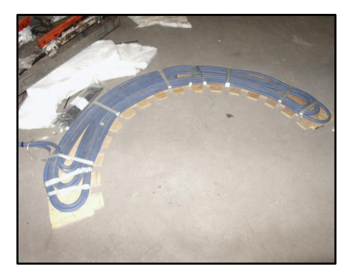
Coils are often configured in creative ways to match the geometry of the part being heated. Since preheat temperature requirements are often less than 400 F (204 C), nonmetallic fixtures such as plywood can be used to secure the coils.
