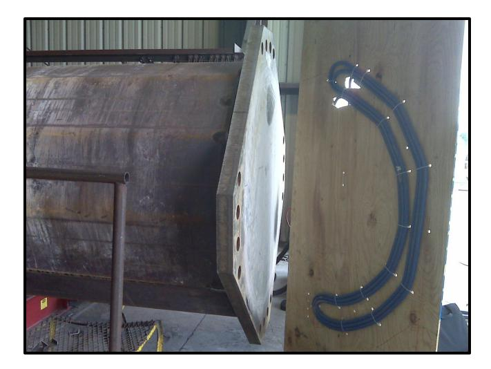
Thick base plates welded to formed steel tubes to fabricate steel poles and towers often require preheat. In this application, the baseplate is heated from the back side while the entire assembly is rotated. Coils are often customized for special applications.
