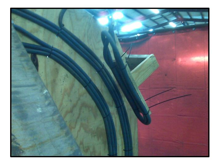
In this view, part of the heating cable is used to make a small coil to heat a portion of the formed tube. Since the tube steel thickness is less than the baseplate thickness, a smaller coil is formed to prevent overheating.
