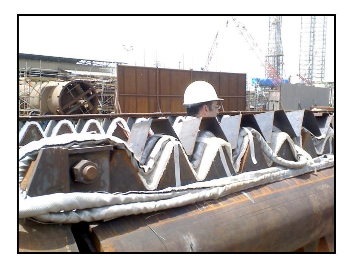
In this application, the heavy teeth of a jack-up riser require preheat prior to welding to a structural pipe. The PROHEAT's liquid-cooled coils can easily follow the contour of many complex geometries.
