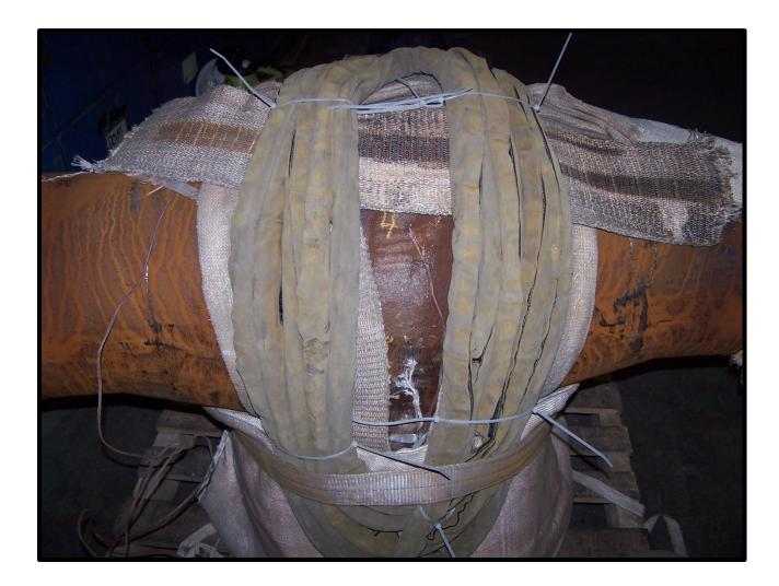
This value body repair application photo illustrates the ability of the coil to be configured in many shapes to match the geometry of the part.
