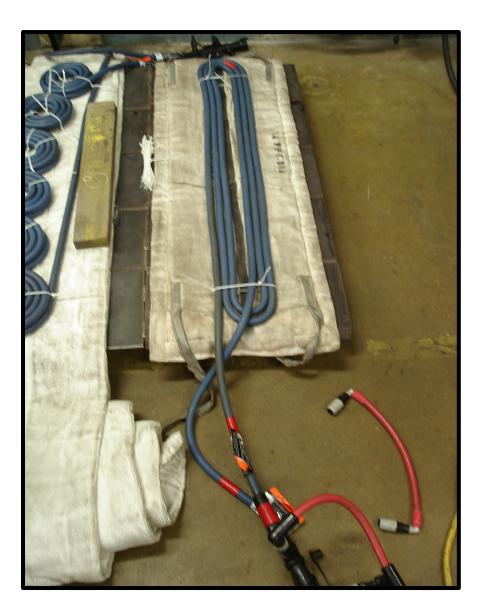
Many coil types can be created with the liquid-cooled heating coils.
