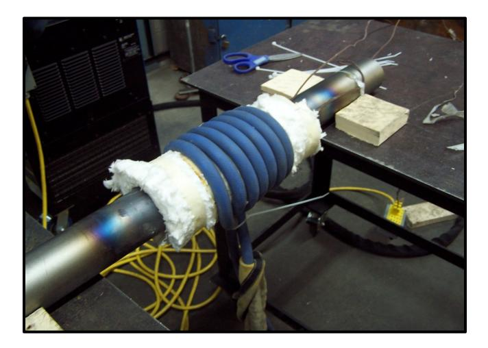
In this small diameter pipe application (app. 75 mm), a test is being conducted to determine the least number of turns required to establish a load sufficient for the PROHEAT to run at a load without faulting. It is very common for the PROHEAT to run at a power level much less than 35 KW for small part heating applications. KAOWOOL should not be used for industrial heating applications.
