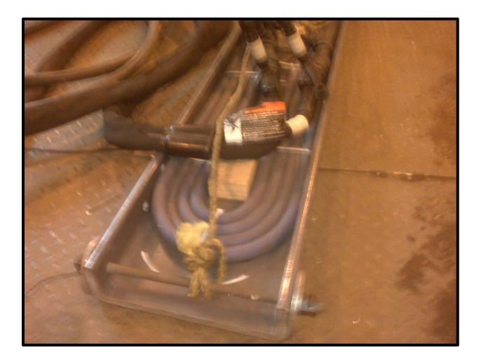
Coils have been successfully used in fixtures designed to move in front of a sub-arc welding torch to enable heating "on-the-fly". In this application, the PROHEAT does not use thermocouples for temperature feedback and control. Instead, the PROHEAT is used in MANUAL mode to control power to the coils in front of the weld. This fixture is a heatresistant, fiberglass channel using carbon-reinforced rods for the axles. The wheels are made out of nonmagnetic stainless steel.
