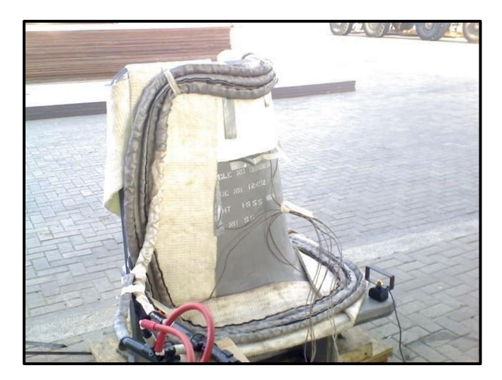
This is a steel casting requiring preheat along its perimeter prior to welding.
