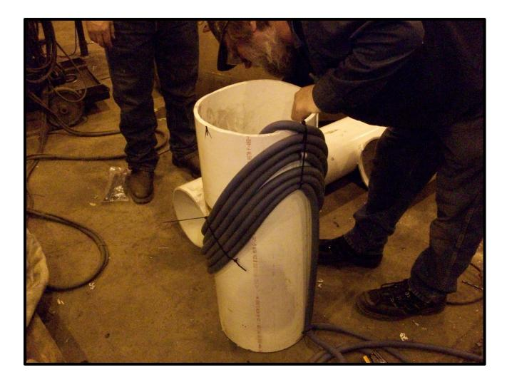
Nonmetallic fixtures are commonly used to secure the flexible induction heating coil to heat various geometries. This coil layout is intended to heat the ID of a pipe segment being welded to a large tank at a skewed angle as shown in the next photo.
