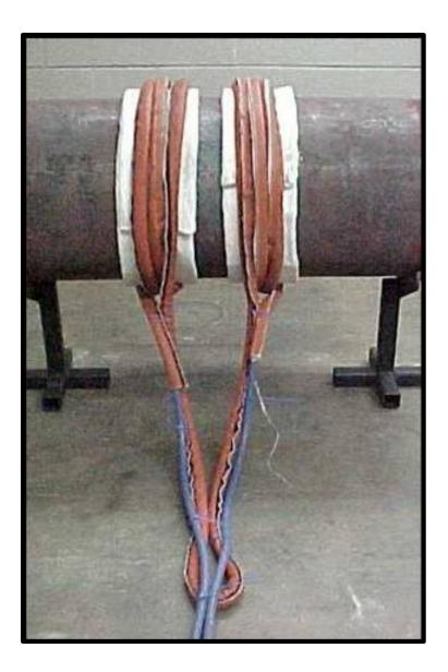
Water cooled induction heating cables are often used for preheat applications. This photo shows the proper coil configuration to heat each side of a weld zone with one cable (with protective cover).
