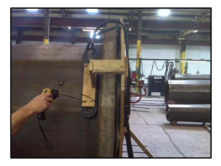
In this view, the coil fixture is in position so that the plate/tube assembly can freely rotate. The steel heats up as it moves past the coils, which are in a fixed position.
