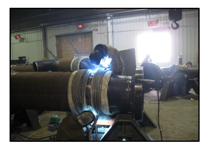
Many fabrication shops require preheat for power plant and process pipe subassembly welding. One coil is used to heat both sides of the weld joint, maintaining preheat throughout the entire weld cycle. The coils themselves do not get hot while energized. Note the new silver preheat covers for the heating cables.
