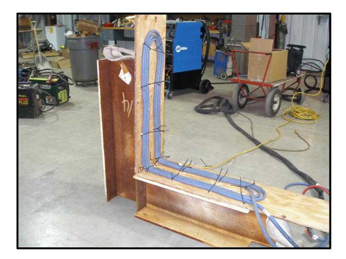
An elongated pancake coil can be used to heat weld seams in flat plate or positioned at an angle as shown here to preheat two I-Beams that are perpendicular to each other. Plywood fixtures are often used for low temperature preheat applications. If you look closely, you will see ½" thick preheat insulation separating the plywood fixture from the steel.
