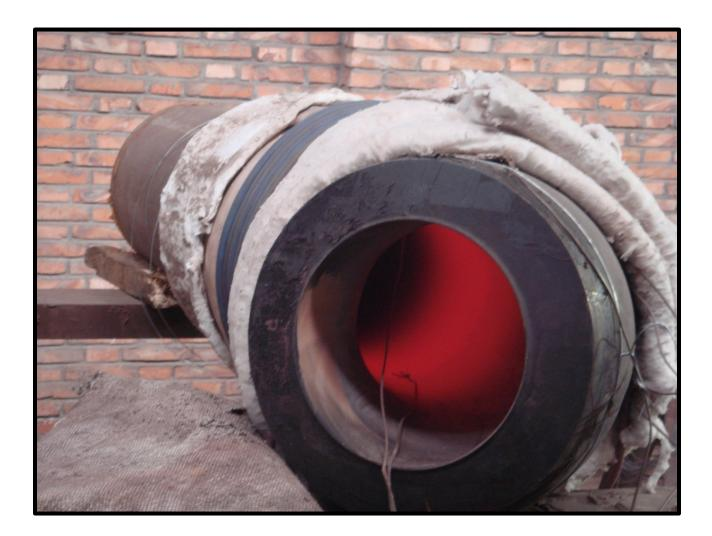
A heavy wall, P92 pipe section is being heated to 1400 F (760 C) in a PROHEAT trial to make sure that the heat soaks through to the ID of the pipe. Note the thermocouple mounted to the ID.
