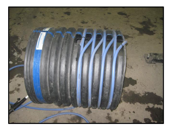
This coil fixture uses a corrugated plastic pipe to help guide and secure a double stack coil used to heat the ID of a heavy wall pipe/flange assembly shown in the next photo. This configuration magnetically coupled with the steel to obtain the full 35 KW output from the PROHEAT.
