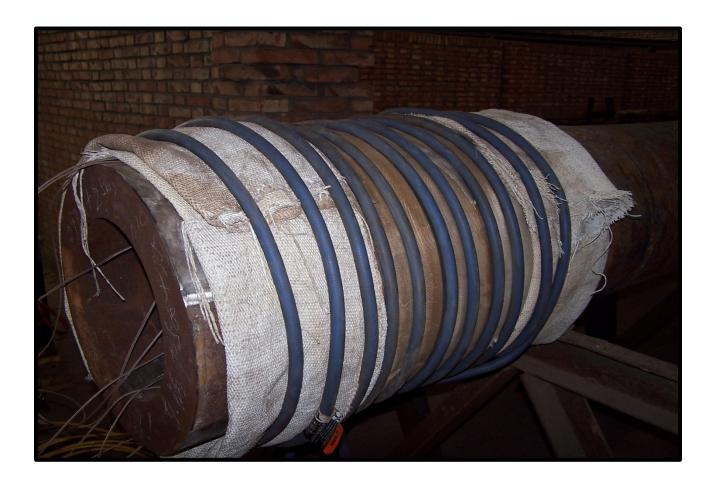
Coils do not have to be right next to each other for every application. Often, the coil is not long enough to span the entire heating zone with coils tightly wound. In this example, the coil is created with a 3" to 4" (75 to 100 mm) gap between the turns. Maximum heating occurs directly under the cable, but fills in evenly between the cables with time.
