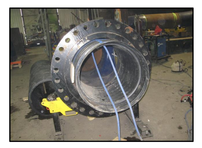
The coil fixture is position on the ID of the pipe/flange assembly, providing preheat from the inside out and unobstructed weld accessibility on the OD. Spacers are used to maintain a uniform air gap between the coil and the ID. Similar coil fixtures are often secured to a stationary stand to permit the part to rotate while welding.
