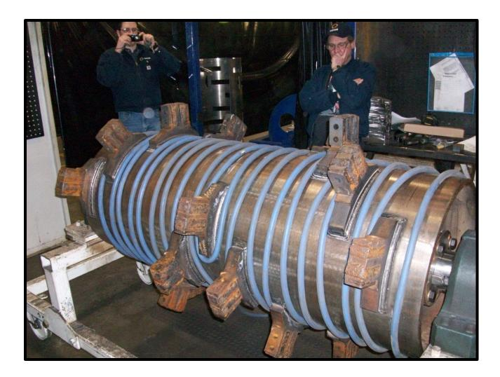
Here, a large spindle used for grinding tree trunks and limbs requires preheat to weld on the "teeth". The customer is considering the coil layout to evenly heat the spindle before adding preheat insulation.
