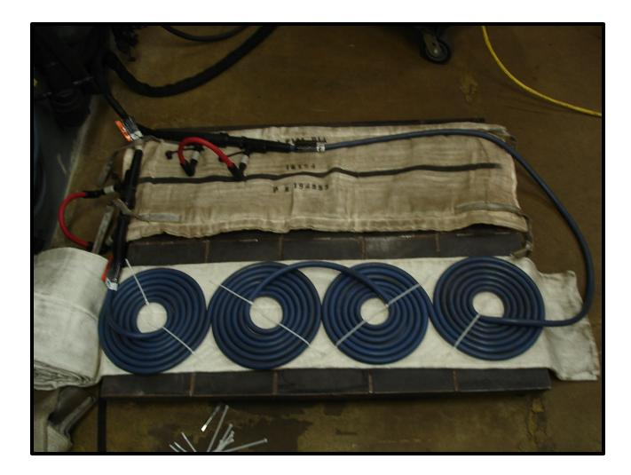
This is another example of a test coil for flat plate or heating "on-thefly". The coil is flexible enough to be able to wind into tight circles for concentrated zonal heating.
