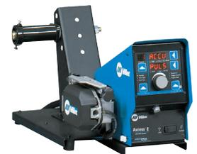
Access E four-drive-roll wire drive feeder is combined with an operator interface, leaving no controls back at the power source. Provides positive feeding for the appropriate preprogrammed wire diameters from 50–1400 IPM, and operates from 40 VDC supplied by Access power source.
