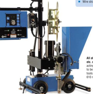
All of the arms, support posts, etc. can be removed with quick acting clamps enabling the carriage to be totally dismantled without tools and easily passed through an 610 mm manhole.
