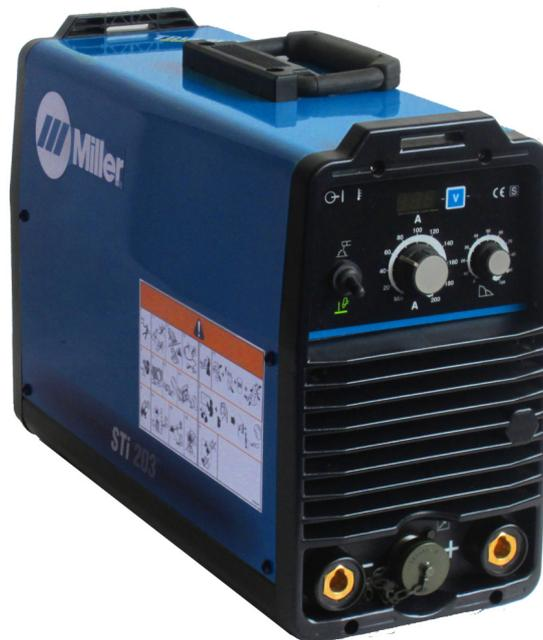
**Adaptive Hot Start<sup>™</sup>** for Stick arc starts, automatically increases the output amperage at the start of a weld should the start require it. Prevents the electrode from sticking and creating an inclusion.
